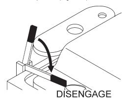
Figure 46. Transmission Engage/Disengage Lever (Disengage Position)
